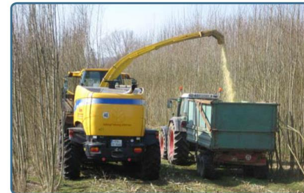
Figure 17. Examples of single pass cut-and-chip system: the harvesting machine cuts and chips the stems and the chips are discharged directly into a tractor-trailer units.
