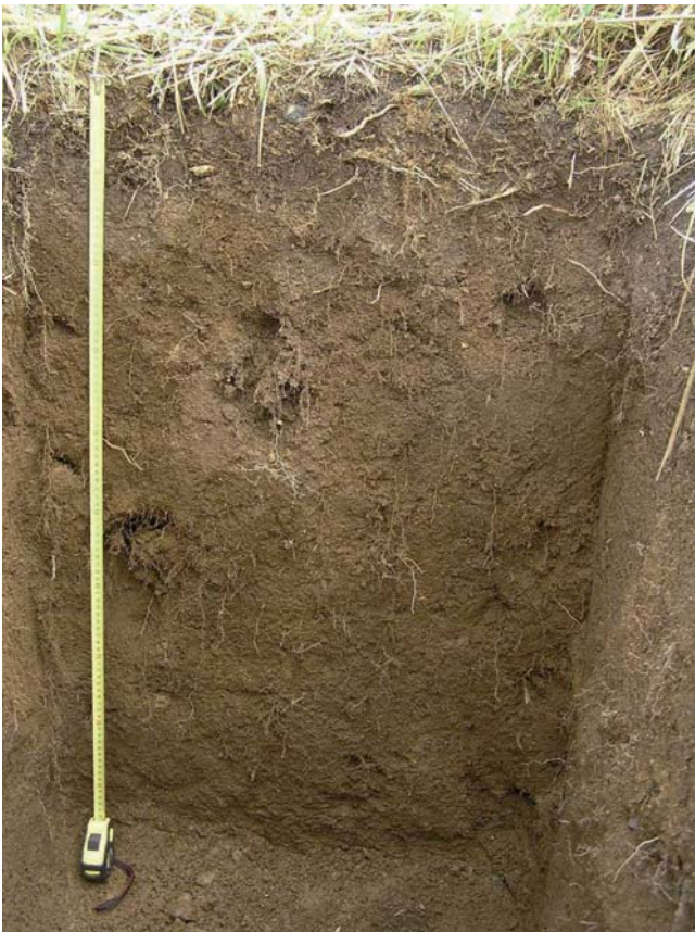
Photo 12. View of the soil profile (depth of 100 cm) at the research site. Good soil structure, absence of coarse rock fragments and rather intensive rooting in deeper horizons of soil are visible
